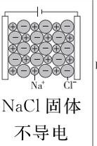
NaCl 固体不导电 |
