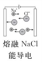
熔融 NaCl 能导电 |
